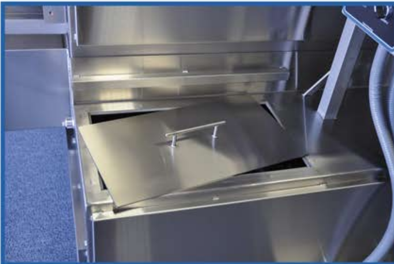
Large tank access cover, directly over sump area of reservoir.
