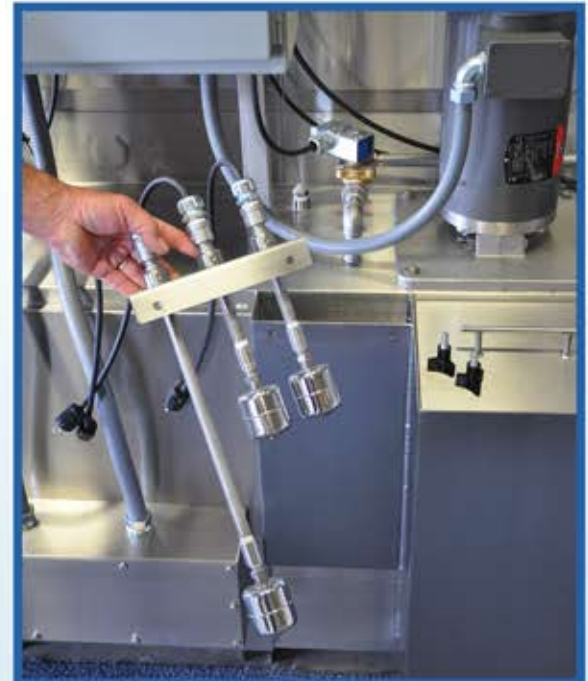
Easily removable float bank for maintenance.
